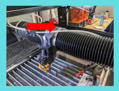
Release the head unit and move it to about 5 mm above the metal slats using the big black knob. Make sure that the head unit does not crash into the slats.
