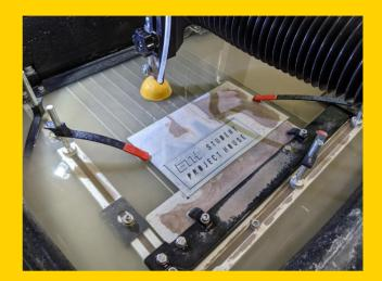
Once more remove the abrasive tube and secure it on top.
